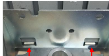
Slide slots onto tabs in bracket
