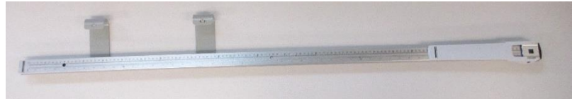
Height Rod with Mounting Brackets
